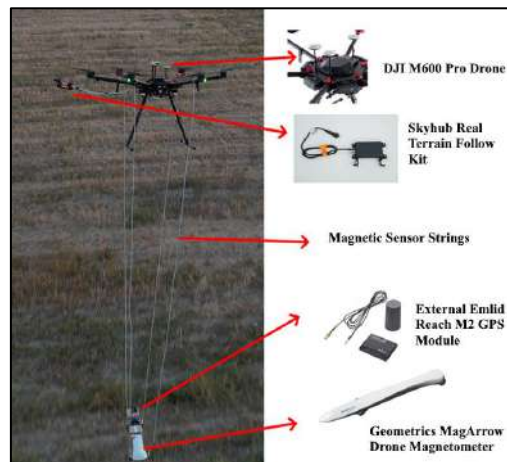
Figure 4. Components of the UAV magnetic system.
