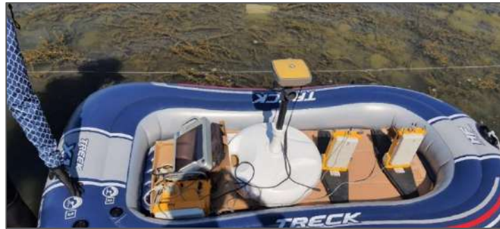
Figure3 GPR measurement setup with 200MHz antenna
