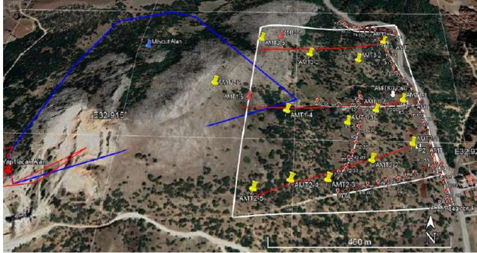
Figure1 Blue polygon: current boundaries of the limestone quarry, white polygon: geophysical study area boundaries, yellow symbols: AMT stations, white lines within the study area: DCR lines, the white down arrow: current water well. The settlement can be seen in the east of the study area.
