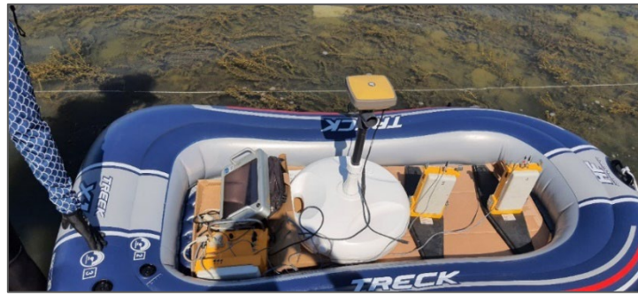
Figure3 GPR measurement setup with 200MHz antenna
